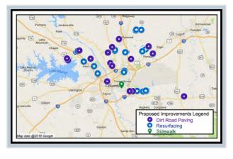
**SCOPE:** The Transportation Improvement Contract 1 includes Resurfacing, Dirt Road Paving and Sidewalk projects. Resurfacing scope: milling, full depth cement stabilization, and/or resurfacing of 23 roads. Sidewalk scope: installation of a 5-foot-wide concrete sidewalk along Capers Avenue. Dirt Roads scope: asphalt paving of 16 dirt roads.
