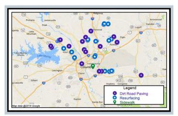
**SCOPE:** The Transportation Improvement Contract 1 includes Resurfacing, Dirt Road Paving and Sidewalk projects. Resurfacing scope: milling, full depth cement stabilization, and/or resurfacing of 21 roads. Sidewalk scope: installation of a 5-foot-wide concrete sidewalk along Capers Avenue. Dirt Roads scope: asphalt paving of 16 dirt roads.
